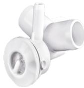
Turbosystem jets are generally located high near upper back and neck. These jets can also be removed for cleaning. To remove this jet for cleaning simply slide a flathead screwdriver between jet cover and tub surface. Carefully turn screwdriver and jet cover comes off. To return jet cover, simply snap into place.
