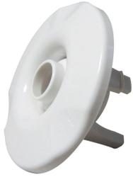
Each jet is adjustable. Simply turn the jet cover left or right and jet flow will adjust up or down. The nozzle inside the jet cover can be adjusted to angle the jet flow in the desired direction. To remove this jet for cleaning simply slide a flathead screwdriver between jet cover and tub surface. Carefully turn screwdriver and jet cover comes off. To return jet cover, simply snap into place.
