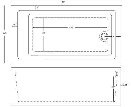
INSTALLATION: Height measurement is inclusive of wood and foam framing. All measurements are +/- 1/2" and are subject to change without notice. Drawing shows recommended pump location as well as approximate location of frame reinforcement legs. Please measure tub before building deck. Data herein supercedes all previous data prior to date shown below.
